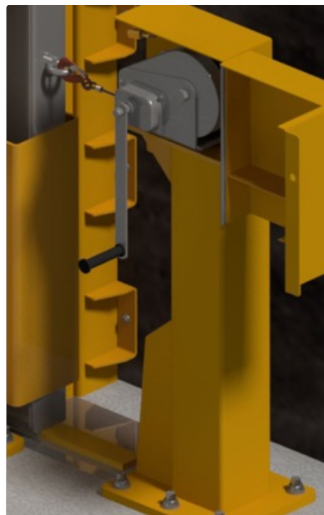
Closing-winch and gearbox mechanism mounted on the gate support posts. A duty and backup hand-pump hydraulic system raises the leaf onto its castors before the winch drives it closed.
